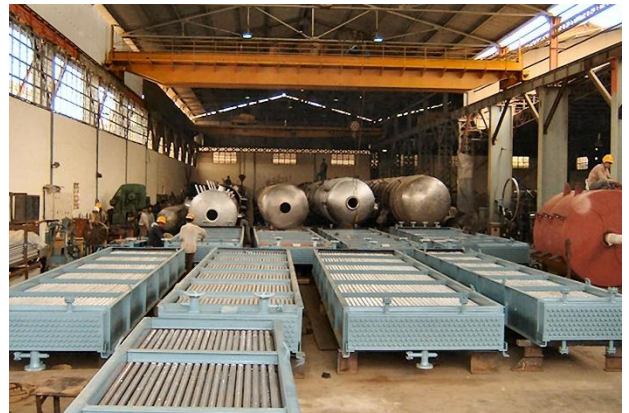
Air Coolers for Oil Refinery
